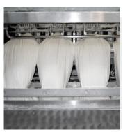
COMBINED WASHING AND MILLING MACHINE Coming from the tradition of quality and the expertise of Biancalani, MILLA is the state of the art solution for combined washing and milling of any type of woollen fabric. Pure-wool or blended, carded or combed, woven or knitted: MILLA is designed for optimal performances ensuring thorough and deep milling on heavy fabrics, and a safe action on lightweight articles, for perfect results, always.
