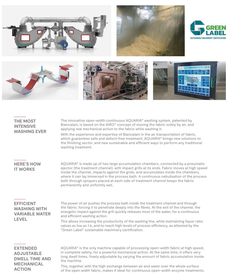
of the open width fabric, makes it ideal for continuous open-width enzyme treatment and provides a fully sustainable approach to bleaching (AQUARIA<sup>®</sup> caustic-free ecobleaching with zero-water discharge), scouring, and fashion effects.
