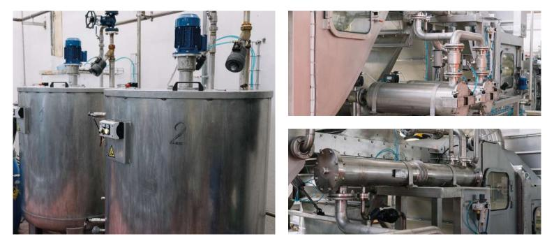
SENSORS AND PROCESS CONTROL Each detail of the process can be controlled with continuity and accuracy, thanks to the availability of several types of sensors and probes. From the level sensors, used to control the water exchange and reintegration, to the temperature probes installed on the recirculation pipes and inside the accumulation chamber of AQUARIA<sup>®</sup>, to optional sensors such as pH, ORP/Redox, and electrical conductivity.
